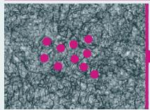
Within the Extended Life series, Allied Filter Systems Ltd is uniquely able to offer a 0.5 micron polyester filter bag. The filter media has a special construction using a blend of micro denier and fine denier fibres, giving the finest filtration results of any needlefelt product available on the market.
