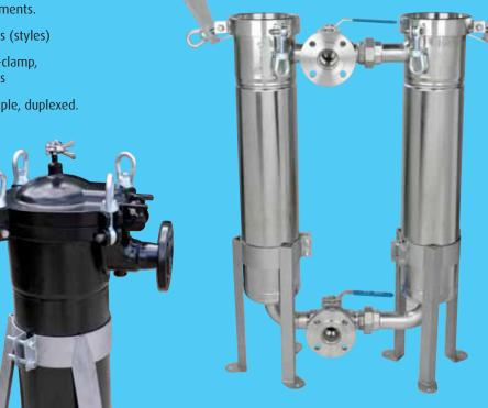
Two RBFP housings manifolded together and fitted with valves to enable use in a continuous process. One filter bag can be changed out whilst the other housing is in use.
